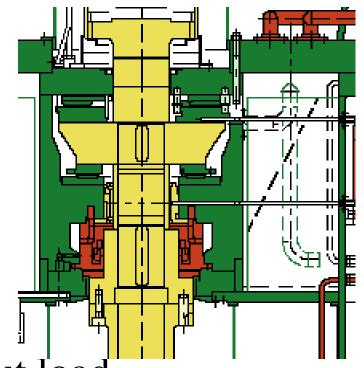
Radial Bearings with/without load single surface multiple surfaces (fixed or tilting pads)
